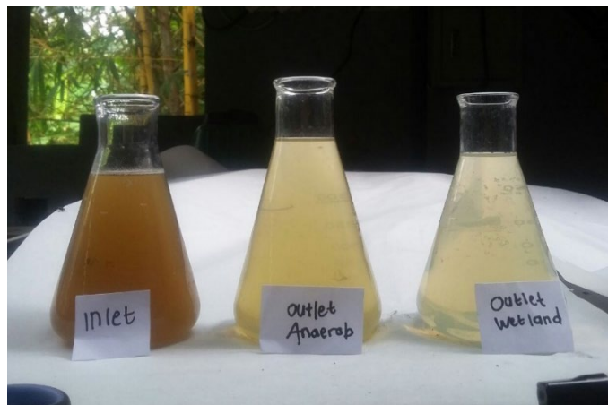
Figure 7. Visual of wastewater from inlet, UAF, and wetland
