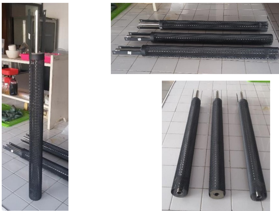
Figure 2. Anode Ti/RuIrO 2 pair configuration and stainless cathode installed in an electrocatalytic reactor
