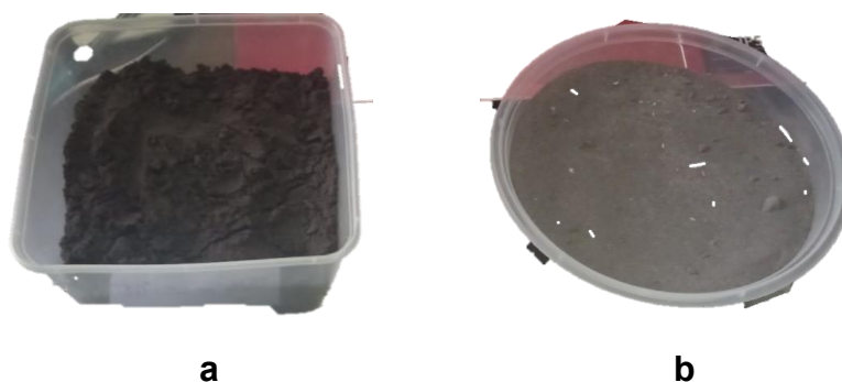
Figure 1. Used catalyst-based activated carbon a) before activation b) after activation
