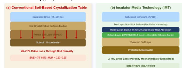
Figure 3. Conceptual comparison between conventional soil-based crystallization tables and Insulator Media Technology (IMT). Sources: ( Allwood & Cullen, 2012 ; Sudarto, 2011 ).
