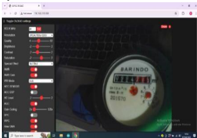
Figure 2. ESP32-CAM live stream output and parameter control interface.
