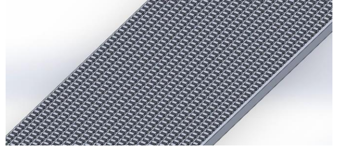
Figure 1. Image of roughing an aluminum surface with rectangular grooves
