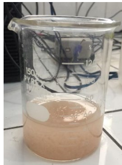
Figure 2. Inactive Aerobic Granular Sludge seed (left). Optical density of inoculum (at 72 h) before added to the MSC system (right).
